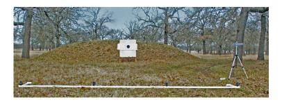
The *fly-over* array has the four microphones lined up on the ground perpendicular to the bullet's expected path. It is easy to deploy. An array 10 feet long will typically detect bullets passing within 10 feet above the array.
