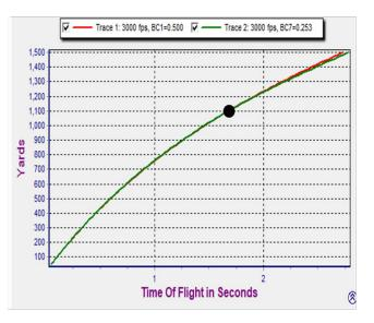
Here are two distance versus time curves using G1 and G7 at the same muzzle velocity. The ballistic coefficients are chosen so that predicted times-offlight match at 1100 yards (velocity near Mach 1.2). The difference in zero-adjust remains less than 0.1 mil out to 1350 yards where the bullet has fallen subsonic.
