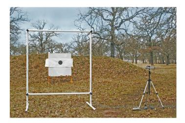
A square *fly-thru* array may be used. The square array provides more reliable scoring, but it is more trouble to set up. The maximum size is 10 feet. Either *fly-thru* or *fly-over* arrays provide excellent time-of-flight measurements.
