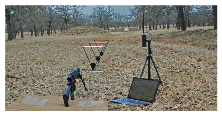
A conventional chronograph measures velocity near the muzzle. The *BC Chrono*<sup>©</sup> System 89 measures both muzzle velocity **and** the time-of-flight from gun to target. An accurate ballistic coefficient requires both measurements using your ammo and your gun.
